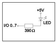
directly. Higher current can be provided by an external transistor circuit. Note that after Power-On resp. in Power-Save-mode all outputs will be at H-level.
